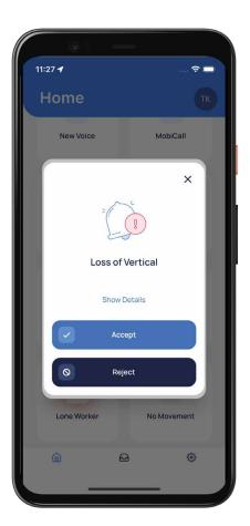
The lone worker protection feature uses location sensors in your smartphone and allows viewing the situation in real-time. If your coworker falls, MobiCall.App is able to determine if the person is laying on the ground and trigger the alarm. To avoid any misunderstandings – the app has a built-in timer which can be used to stop alarms if the event has occurred accidently.
